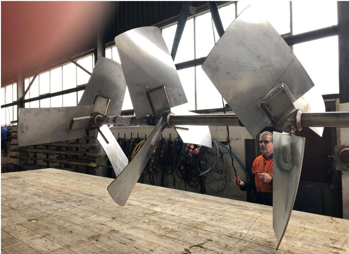
20 Cube Yoghurt Mixer Shaft and Impellers being Loaded onto Truck to go to Metal Polishers
