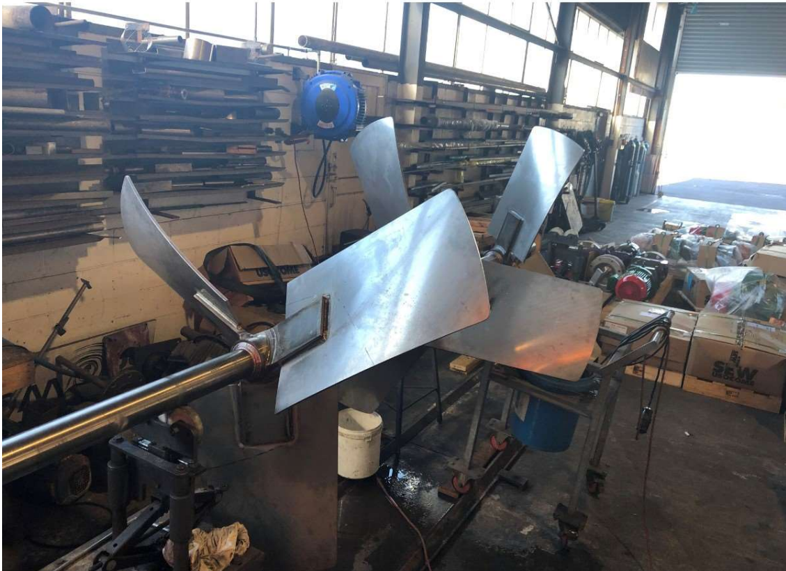
20 Cube Yoghurt Mixer Shaft and Impellers on Straightening Jig
