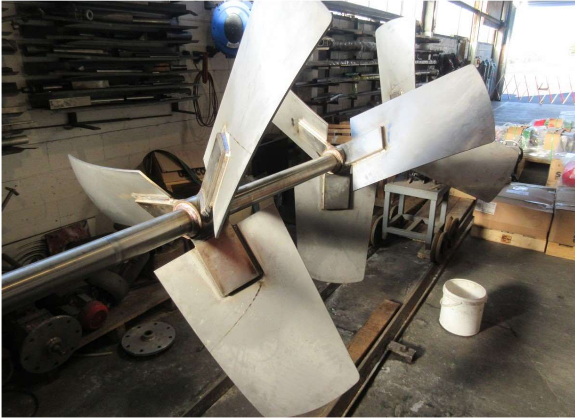
20 Cube Yoghurt Mixer Shaft and Impellers now Straightened Ready for Polishing
