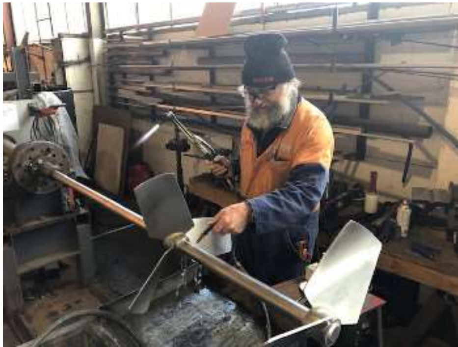
Brian at Work with Oxy-Acetylene Torch and Cooling Water Nozzle
