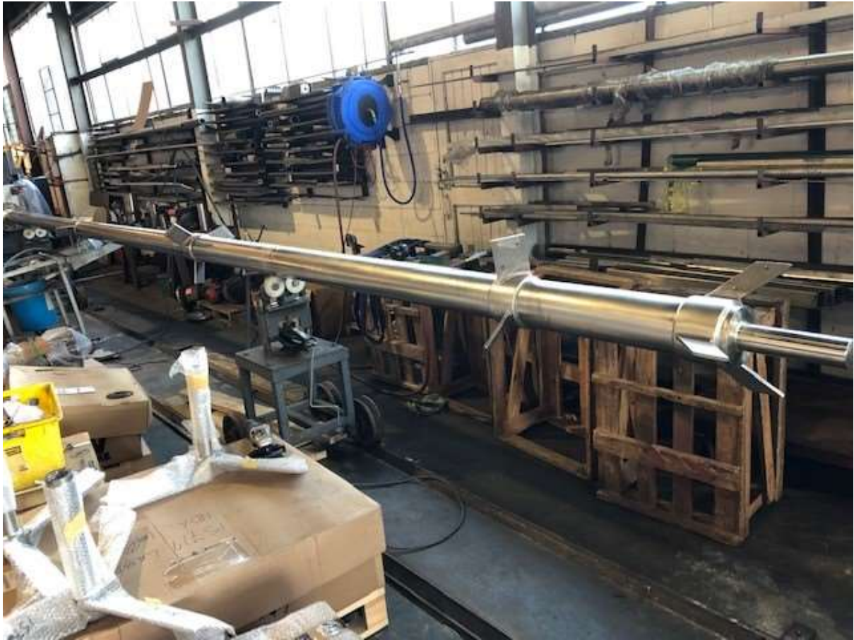
Shaft Straightening Jig with long Hollow Shaft ready to be Straightened
