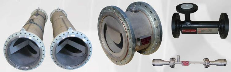
Static mixers are typically used for mixing two or more continuous streams of liquids or gases together and to disperse gas into liquids. They can also be used to ensure a uniform thermal profile within the pipeline. Applications include diluting acids, pH correction, dissolving air into a DAF system, chemical dosing in water treatment, geothermal brine pH balancing and flocculant dosing. Approved for use in ACC Watercare Material Supply Standard.
